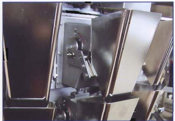
MultiWeigh® "Direct-Drive System", steppermotor operated hoppergates
